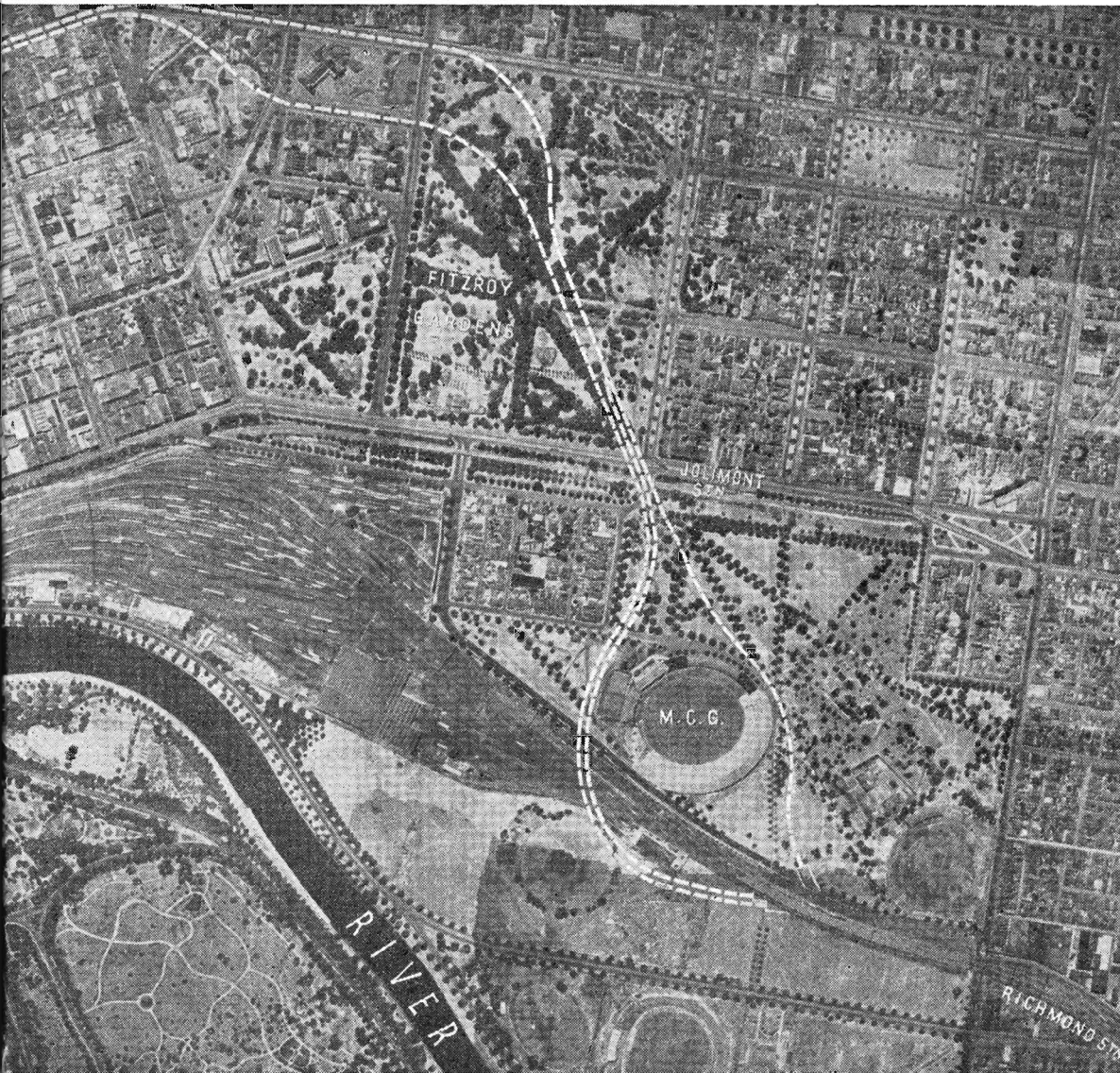
Proposed new railway from Richmond Station to the Flagstaff Gardens and connecting also with the present service at by a white dotted line.
